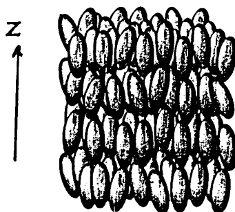
Fig. 5 Illustrating the structure of a smectic A mesophase.
